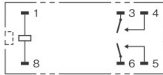
Terminal Assignment Internal Connections (BOTTOM VIEW)
